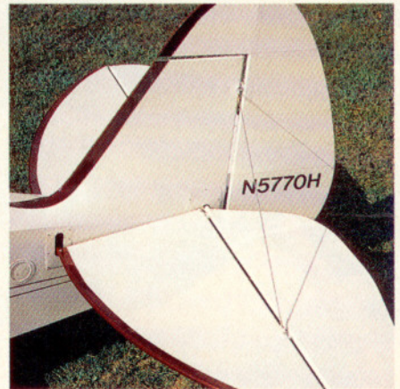
The Clipper's Lycoming O-235 engine is straightforward to maintain (top left) and the cargo area is roomy enough for a weekend's worth of baggage (left). The Clipper's aileron cables are exposed (top center) and the tail (above) recalls that of the Piper Cub, with wire supports for the horizontal stabilizer.
